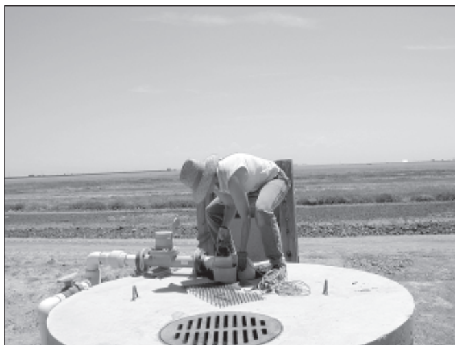
Water monitoring samples are taken from a sump at the Red Rock Ranch near Five Points.
