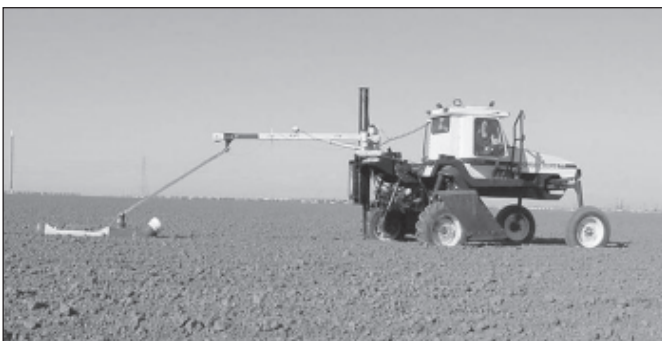
Figure 1. EM-38 survey equipment
